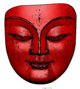
7 Click the Delete button on the Main toolbar to delete the cloud and display the mesh.
