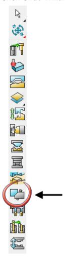
The **Slide Wizard** starts. This wizard is used to design the mechanism that removes the slide core and adds it to the mold base.
