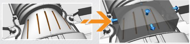
Extract the burn region from the workpiece using a Solid Core. Select the faces that surround the region to be extracted and then choose an appropriate blank, either from major suppliers such as EROWA, or your own user-defined library. The blank can be adjusted dynamically to your exact requirement using intuitive drag handles. The new core, extracted directly from the workpiece, can be modified if necessary using any combination of surface, solid or Direct Modelling techniques.
